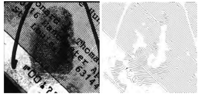
Fig. 13. Poor quality of the latent fingerprint images makes it difficult to reliably extract features from latents. The image on the left is a poor quality latent in which the ridge pattern of interest is smudged and occluded by the presence of structured noise (text, lines, etc.). On the right is shown the ridge skeleton extracted by a commercial fingerprint SDK from the image on the left. Since the SDK used for extracting the above ridge skeleton is not specifically designed for processing latent prints, it fails to extract the correct fingerprint ridges from the latent.
