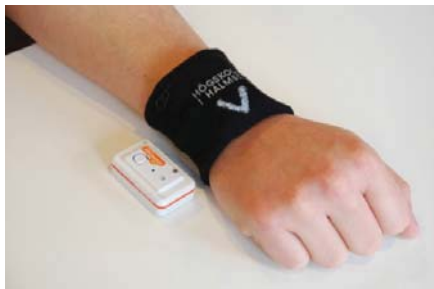
Figure 3. The Shimmer is placed inside a wristband. One platform is worn on each wrist by the instructor in the game design and by the player during the game play.
