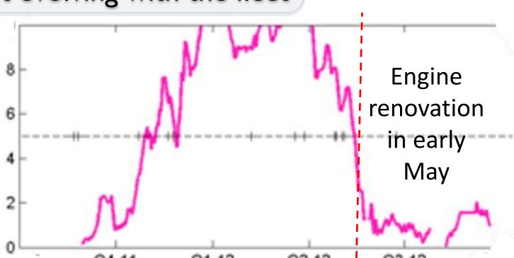
When one of the group members starts to deviate from the normal behaviour, it is reflected in the differences between data models obtained from individual vehicles.
