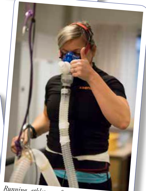
Running athlete performing a maximal lactate test on a treadmill. Data of lactate, oxygen consumption, muscle activity, acceleration and feet pressure is captured during an incremental running test. The data analysis aims to predict fatigue from indirect measurements.
