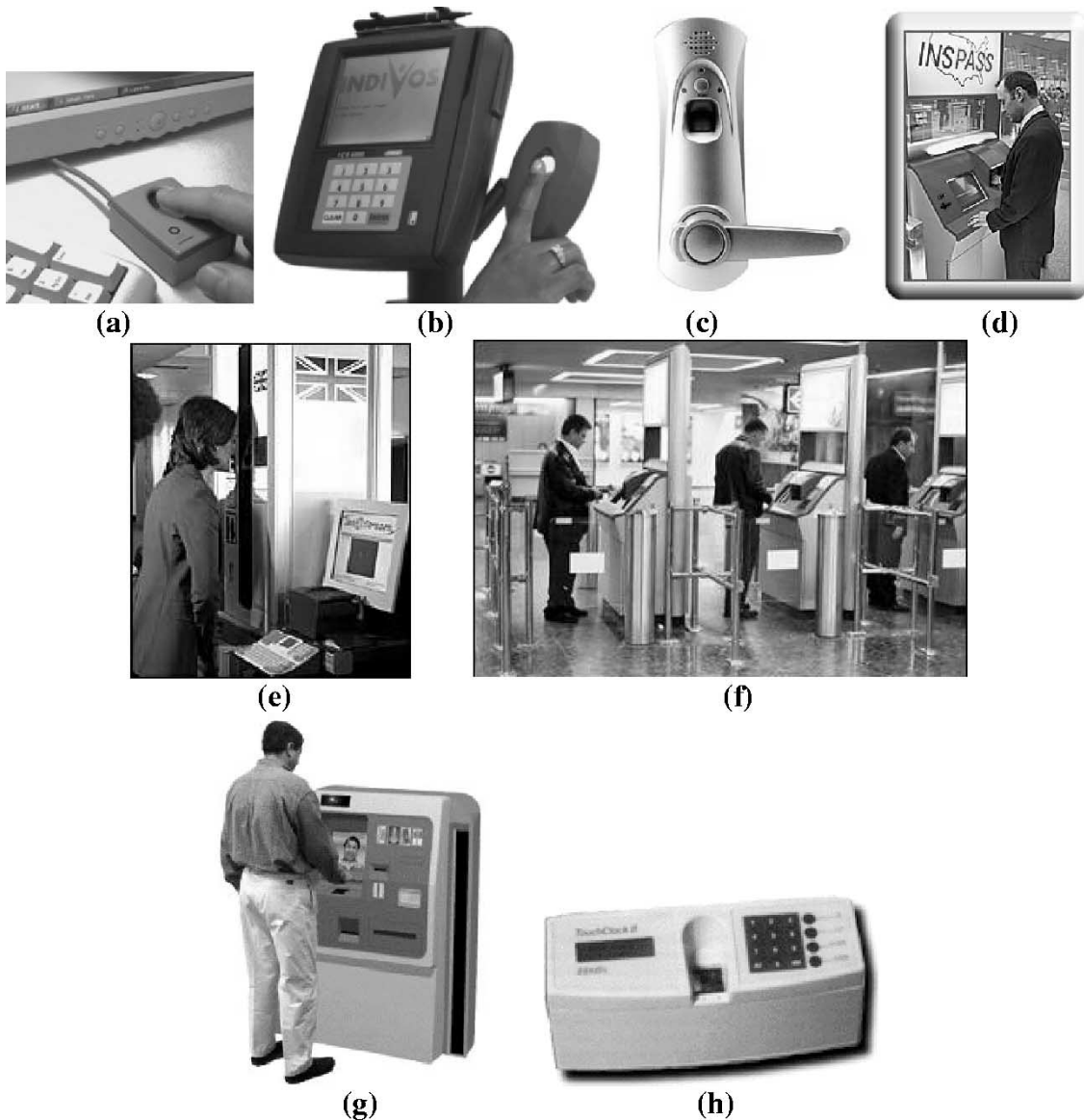
Fig. 4. Examples of biometric application. (a) Fingerprint verification system manufactured by Digital Persona, Inc., is used for computer and network login. (b) Fingerprint-based point of sale (POS) terminal manufactured by Indivos, Inc., that verifies the customers before charging their credit cards and speeds up payment in retail shops, restaurants and cafeterias. (c) Fingerprint-based door lock manufactured by BioThentica Corporation used to restrict access to premises is shown. (d) Immigration and naturalization service accelerated service system (INSPASS), which is installed at major airports in the U.S., is based on hand geometry verification technology developed by Recognition Systems, Inc., and significantly reduces the immigration processing time. (e) Border passage system using iris recognition at London's Heathrow airport. (f) Ben Gurion airport in Tel Aviv (Israel) uses Express Card entry kiosks fitted with hand geometry systems for security and immigration. (g) The FacePass system from Viisage is used in POS verification applications like ATMs, therefore obviating the need for PINs. (h) The Identix TouchClock fingerprint system is used in time and attendance applications.
