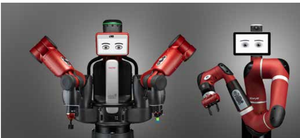
Robots such as Baxter (left) and Sawyer (right) can use a rich variety of sensory and behavioral modalities to seek to recognize human actions and intentions and behave in a way which appears safe and transparent. For SIDUS AIR, a Baxter with a Ridgeback mobile base has been procured.
