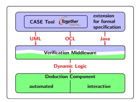
Fig. 1. The architecture of the KeY system
