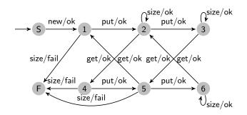
Figure 4: Failure model of the queue of size 2.
