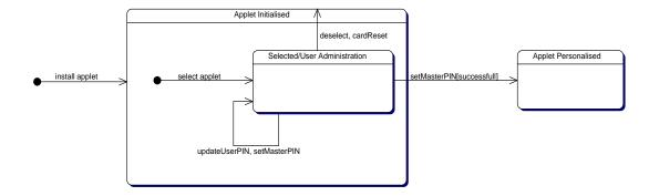
Fig. 2 Command states in the initialised life cycle state
