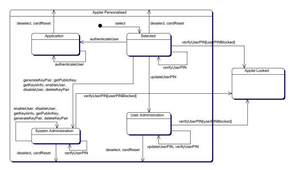
Fig. 3 Command states in the personalised life cycle state
