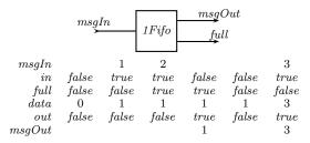
Figure 2. Sample behavior of a 1-place buffer
