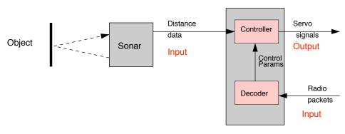
All messages/events are asynchronous! Either generated by the CPU or by the sonar hw or by the communication hardware.
